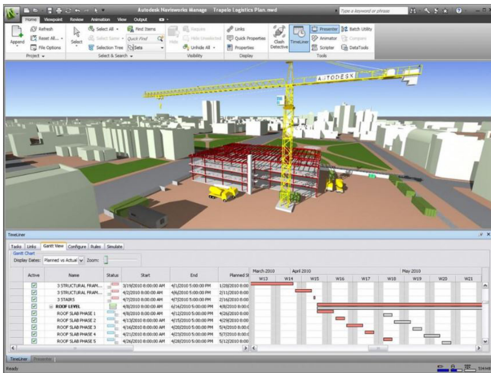
Figure 83: Example of a construction programme. (Autodesk)
