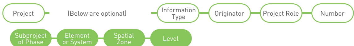
Figure 28: Container identifications. (DCT)
